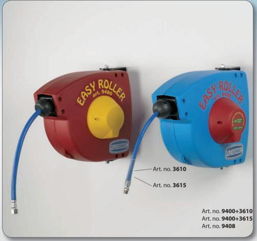
Automatic rewind, spring-driven hose reel, with plastic enclosure (made of nylon and polypropylene) and pivoting wall bracket, suitable for the use with compressed air and water (temperature range:  $-10^{\circ}\text{C} - +60^{\circ}\text{C}$ ) and for hoses of 8 x 12 mm (or 10 x 14 mm) with a max. length of 15 m (or 10 m). Inlet connection air: 1/4" BSP. Max working pressure: 20 bar.
